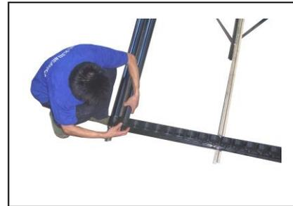
**Screw the cover back into tube holder**
